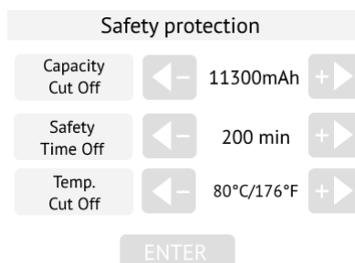
Safety protection settings
