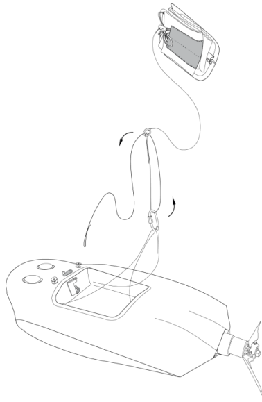
Short static line end turning into the ring of detaching system
