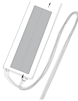
Putting the rigging lines into the pocket
